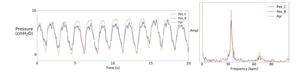
Power spectral analysis of esophageal and pleural pressure signals. The frequency spectra (right) and esophageal pressure signals (left) of both air-filled catheter and balloon catheter revealed concordant predominant respiratory component (large peak at 33 bpm) but also cardiogenic noise from heart rate component (second peak at 80 bpm). Pleural pressure curve and superposition of the three curves with their spectra are shown
